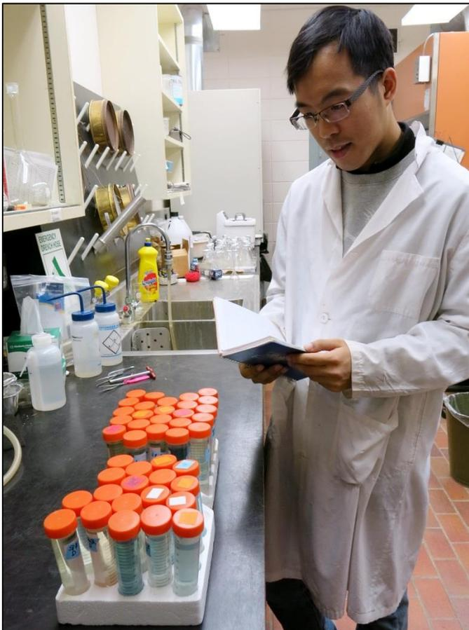
**Figure 2 (Left).** Checking samples of laboratory-based nitrification assays of stream sediments. In case the sample colour is of interest, darker blue indicate higher total extractable ammonium concentrations in the sample.
